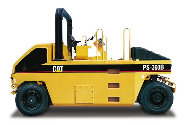
The PS-360B is a pneumatic roller that not only generates high-production results but also is versatile. Its versatility comes from the large and varied ballast capabilities. This allows the PS-360B to be effective on a wide range of applications including soil, asphalt, chip and seal, reclamation, and stabilization.
