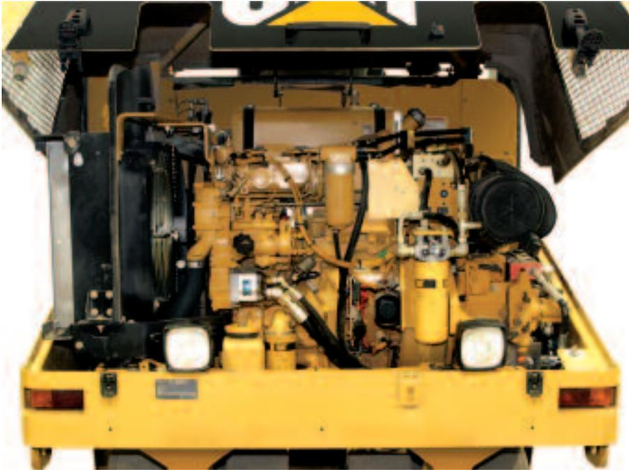
**Large engine enclosure** pivots upward for access to engine.
