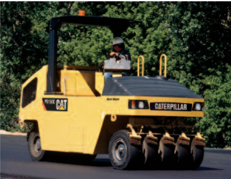
**Maximum operating weight of 17 137 kg (38,000 lb)** increases versatility for working on thick lifts.
